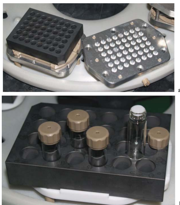
Fig. 1 (a) A 48-position silicon carbide plate; (b) A 24-position silicon carbide plate capable of holding standard glass vials.
